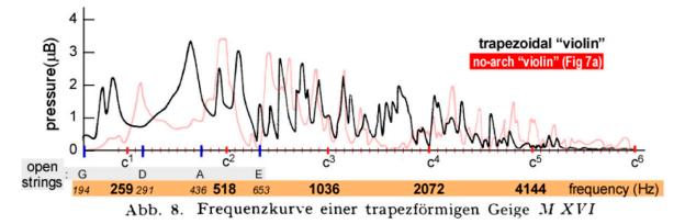
Figure 8. Frequency response of trapezoidal violin M XVI [with superimposed no-arch "violin" from Fig 7a.]
