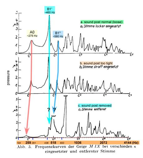
Figure 5. Frequency response of violin M IX with varied inserted and removed sound posts [(a) normal (loose), (b) too tight, and (c) removed; note damping decrease for the too-tight sound post].
