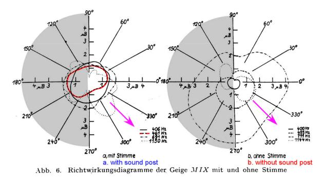
*Figure 6. Radiation patterns for violin M IX with and without a sound post.* [B1<sup>-</sup> *in red; back hemisphere shaded; arrow at 315° in the direction of audience*].
