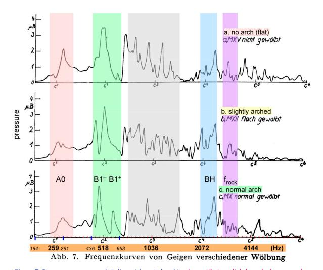
Figure 7. Frequency response of violins with varied arching [none (flat) to slightly arched to normal arch; curves in Fig. 7 all suggest the presence of a sound post; BH and  $f_{rock}$  regions shown shaded, but not sure about bridge properties.]
