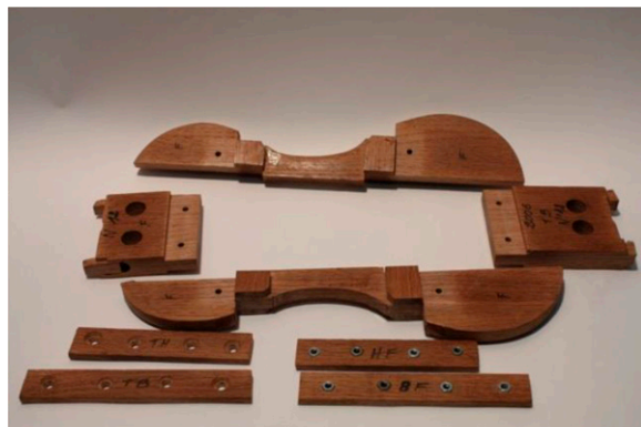
Figure 17. End collapse mold exploded [5].
