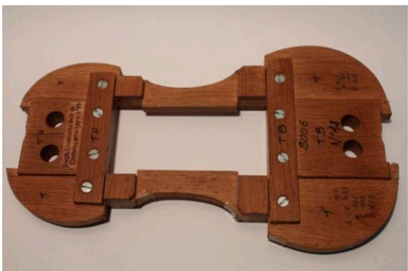
Figure 16. Mold with end collapse [5].
