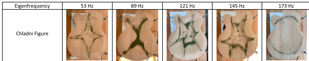
Figure 14. Chladni figures of the archtop guitar free plate, standard graduation. The eigenfrequencies correspond to Fig. 8.
