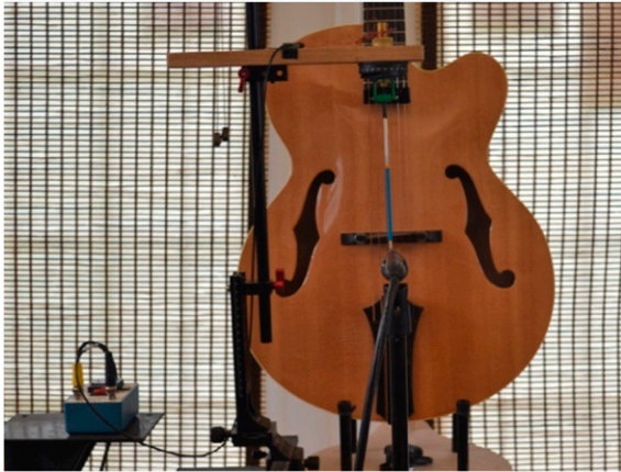
Figure 18. The impulse measurement rig adapted for guitar. Pictured with microphone for near-field radiation measurements.
